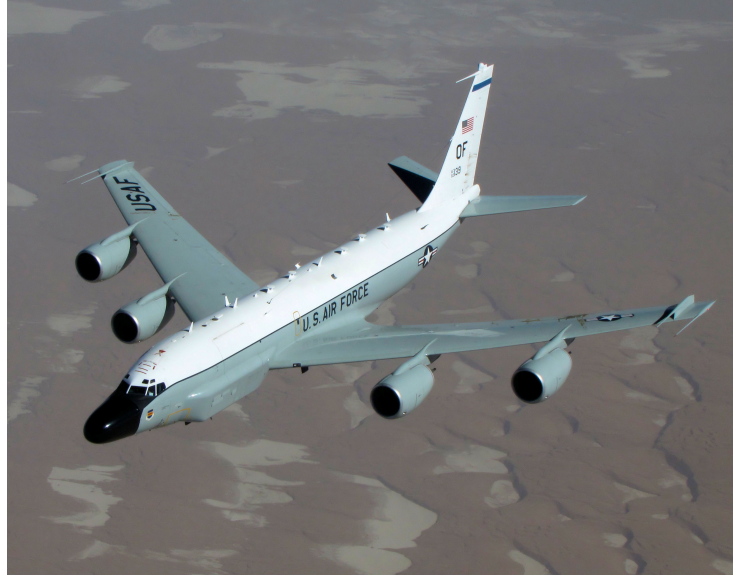
Figure 1.1: RC-135 airframe considered for an airborne high frequency direction finding antenna system. [1]
